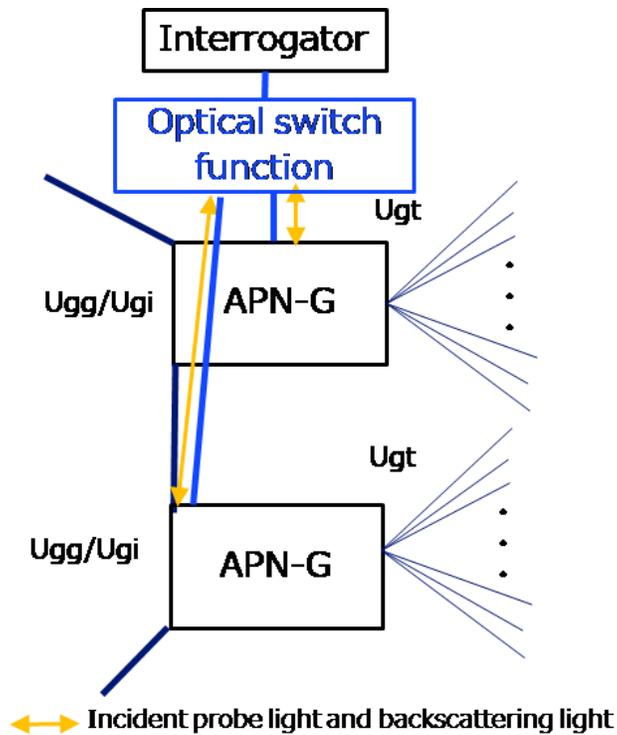
Figure 4-3 External switch dedicated to fiber sensing in the first stage for selecting each APN-G
