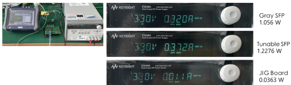
Figure 11 SFP Power consumption measurement and results
