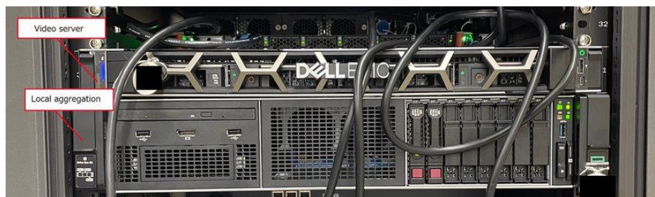
Figure 5-2: The video server and the local aggregation node located in NTT Yokosuka R&D Center
