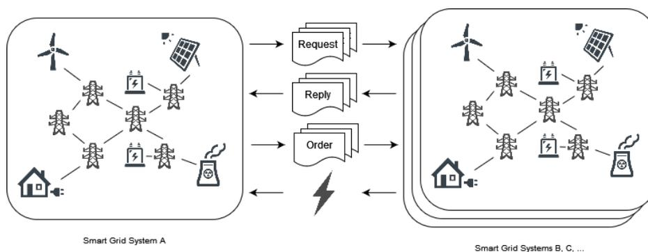
Figure B-13: Direct coordination-based power interchange mechanism among multiple Smart Grids
