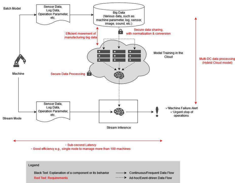
Figure A-9: Intelligent Machine Failure Prediction System
