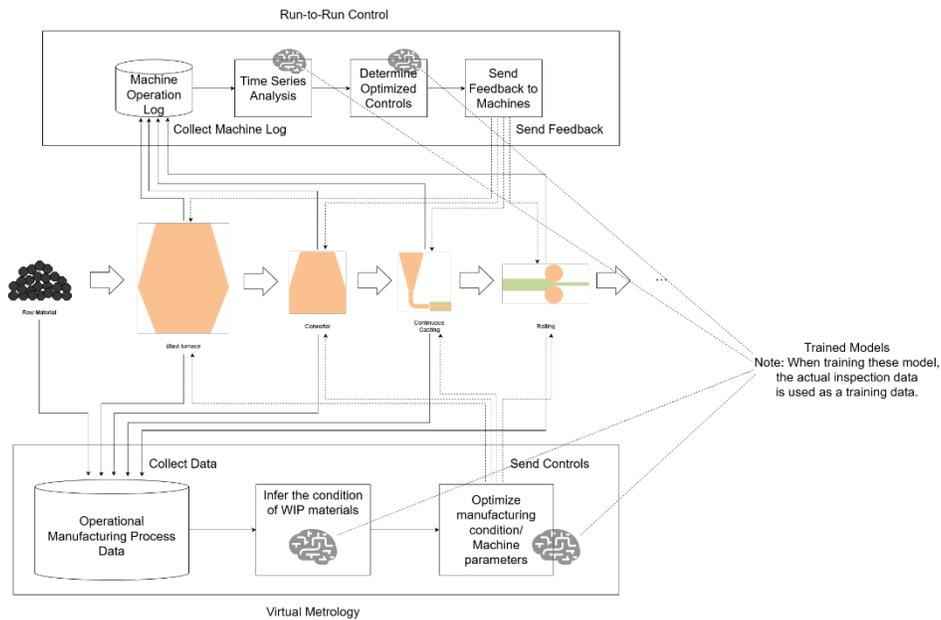
Figure A-10: Intelligent Manufacturing Process Controls
