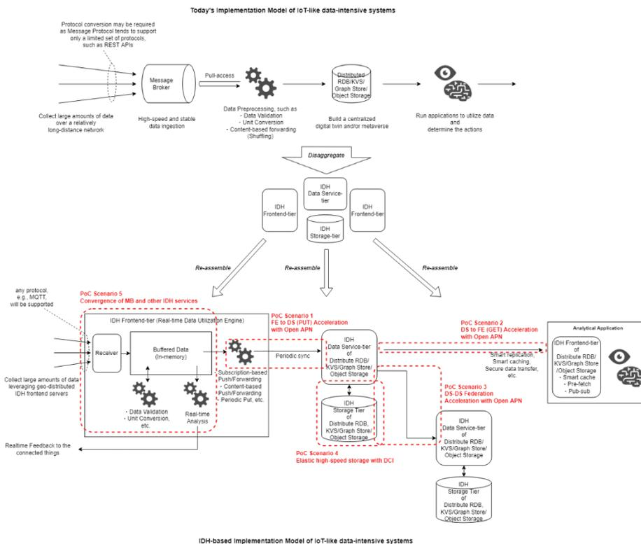
Figure 4-1-2: Devising a new implementation model and PoC scenario mapping
