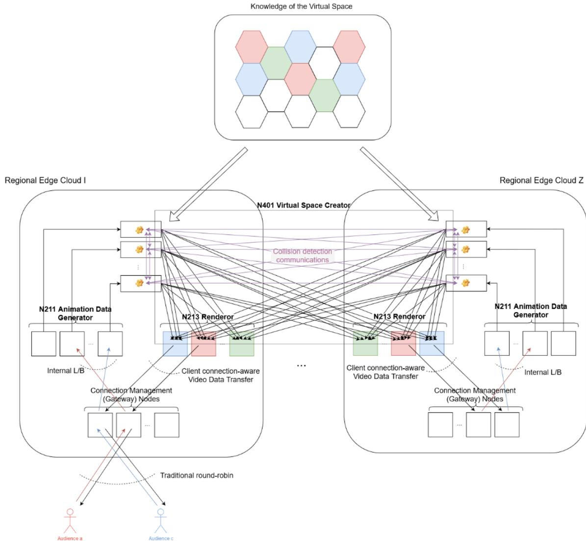
Figure C.1-1: Geo-Distributed Implementation of the Virtual Space Creator
