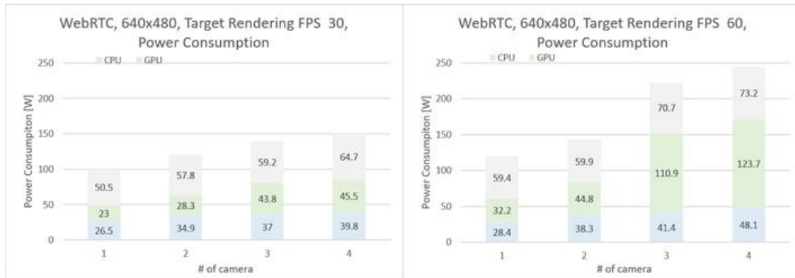
Figure 8.5-1: WebRTC Renderer Power Consumption, 60/30fps
