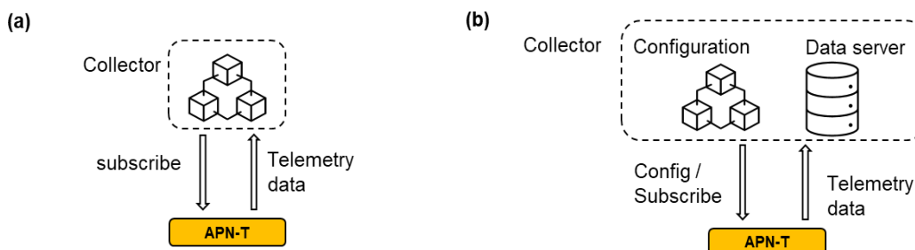
Figure 5.5-3: Streaming Telemetry and Two Collector Configurations
