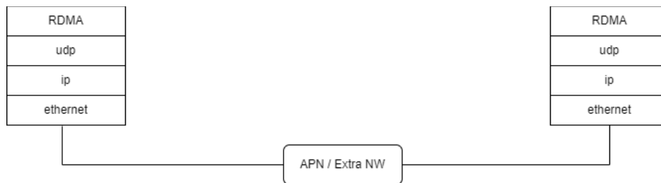
Figure A-19: Protocol Stack for RDMA (RoCE v2)
