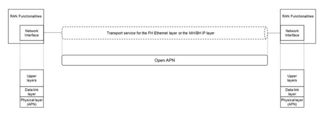
Figure 7 RAN deployment scenario with direct path over APN
