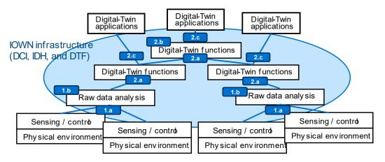
Figure 14 Implementation of the digital twin functions.
